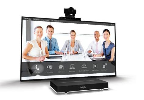
The Avaya Scopia<sup>®</sup> XT5000 provides exceptional video, audio, and data quality along with ease-of-use designed to make users successful. The XT5000 incorporates dual 1080p/60fps live video and content, HD audio, simultaneous H.264 High Profile and Scalable Video Coding (SVC), and multi-party calling. The PTZ camera, supporting 1080p/60fps, offers 10x optical zoom (40x digital) and wide-angle capability for viewing details and an entire group.
